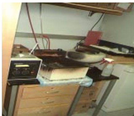
Heat generating equipment in too close proximity to one another, view 2
