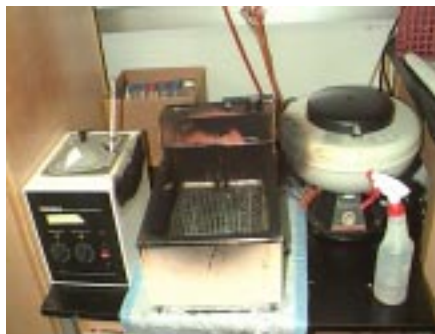
Heat generating equipment in too close proximity to one another, view 1
